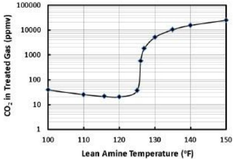
**Figure 6 Extreme Sensitivity to Lean Amine Temperature in an LNG Absorber**
