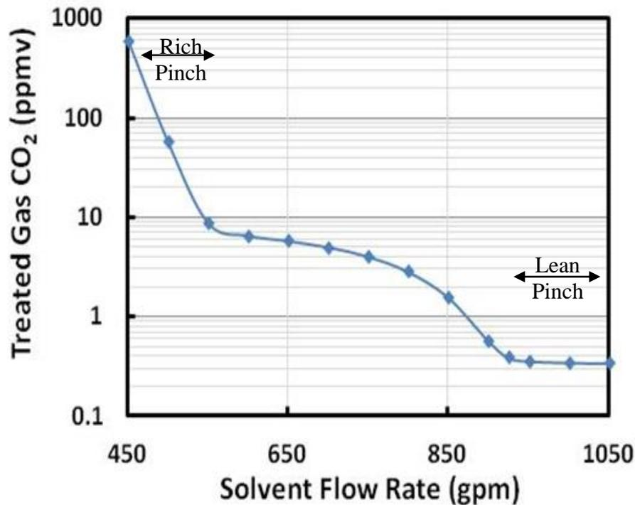
**Figure 1 Performance of a Packed LNG Absorber with 0.015 Lean Loading**
