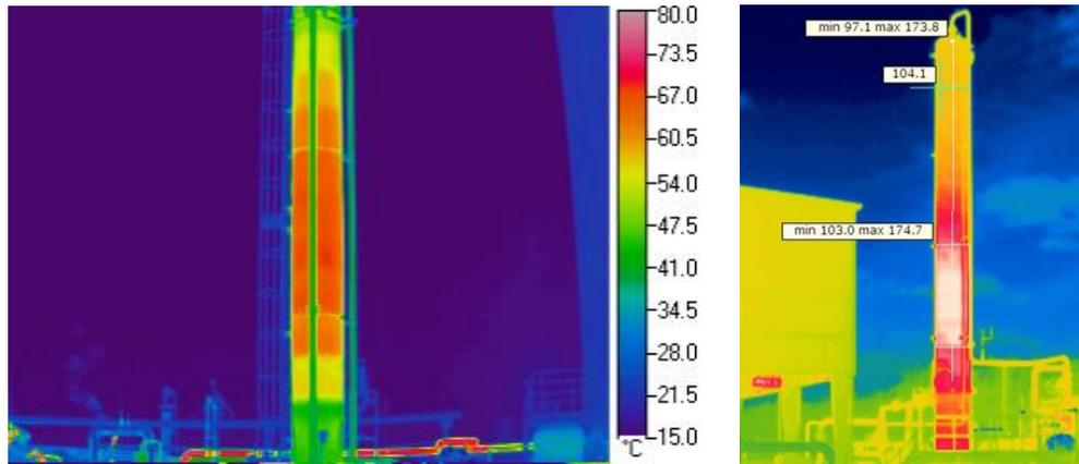
**Figure 7 Infrared Scan of Contactor Profiles with Broad Bulge and Bottom Bulge**
