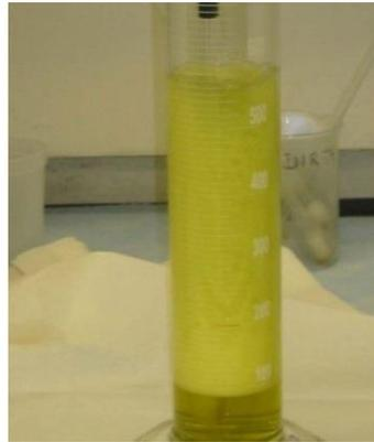
**Figure 3 Foam Test of an Amine Sample following Settling**
