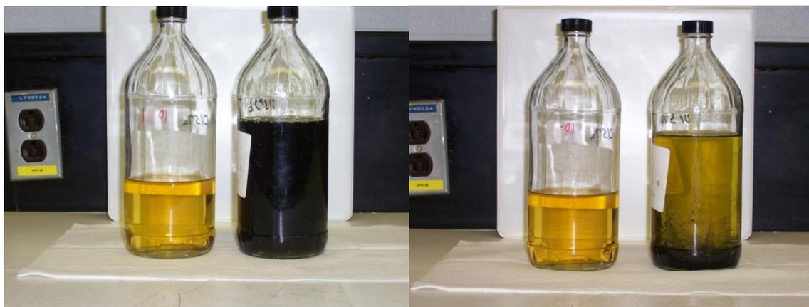
**Figure 2 Amine Samples immediately after sampling (L) and after settling (R)**
