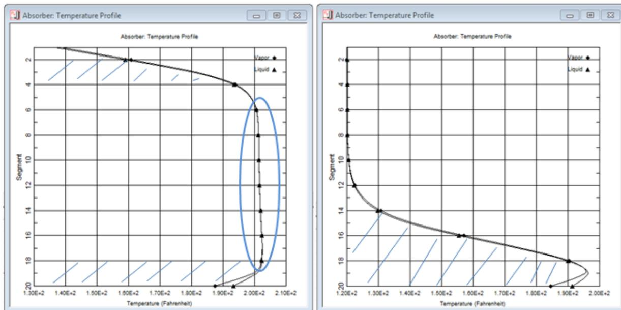
**Figure 5 Bulge Pinched and Lean-end Pinched Temperature Profiles**
