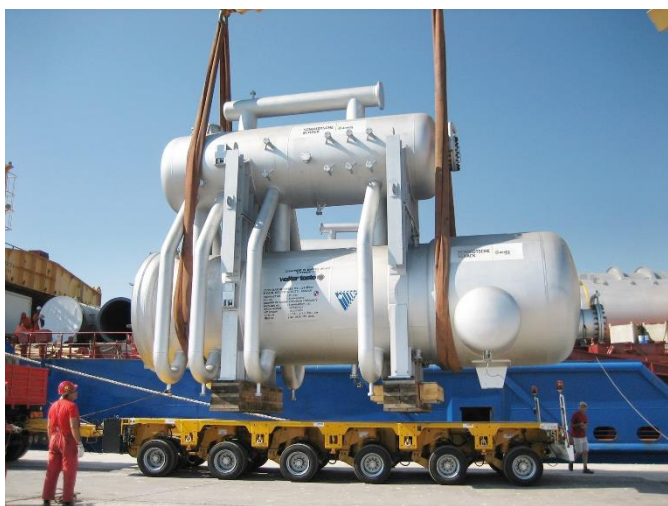
Figure 1 Waste Heat Boiler (courtesy Schmidtsche Schack, Düsseldorf)
