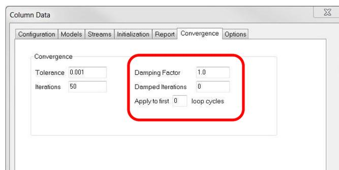
Figure 1. ProTreat Column Convergence Tab
