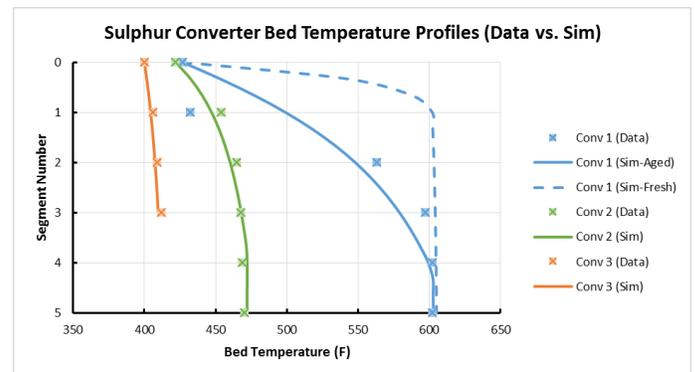
Figure 3: Temperature Profiles from Operating Plant vs. Simulation Predicted Temperature Profiles.
