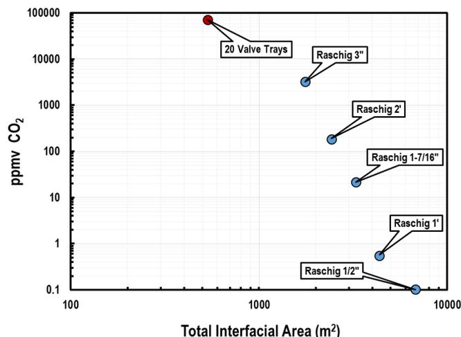
**Figure 1** CO<sub>2</sub> Removal with a Piperazine Activated MDEA Solvent. Performance Depends Heavily on Tower Internals. Note log Scales
