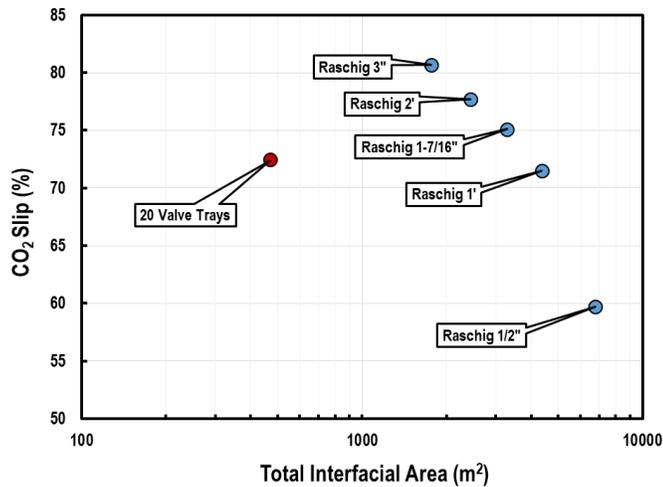
**Figure 2 CO<sub>2</sub> Slip Using MDEA Solvent in a Selective Treating Application**
