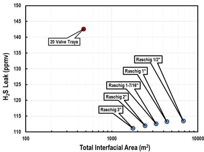
**Figure 3 H<sub>2</sub>S Removal Using MDEA Solvent in a Selective Treating Application**
